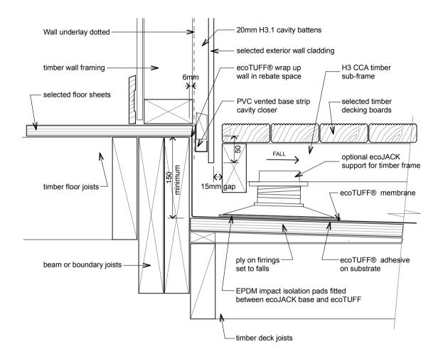
ecoT30 - timber raft floating deck-wall detail - type 2
