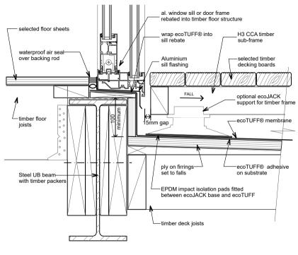
ecoT32 - timber raft floating deck-threshold detail - type 2 Revision: 18 July 2014
