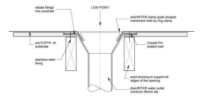
ecoT14 - drainRITE® Water Outlet 1 - ring clamped
