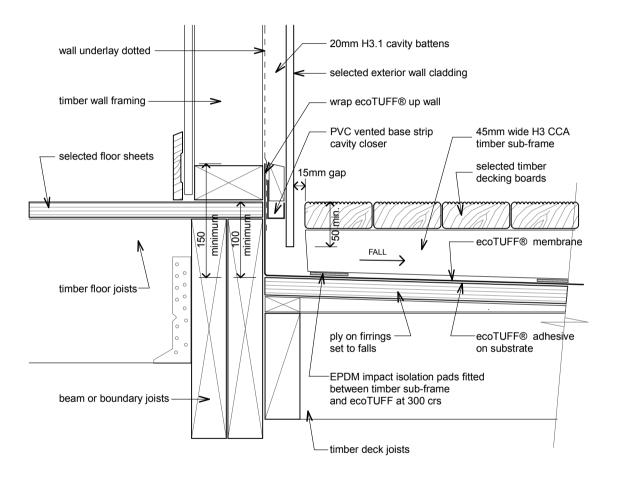
ecoT29 - timber raft floating deck-wall detail - type 1
