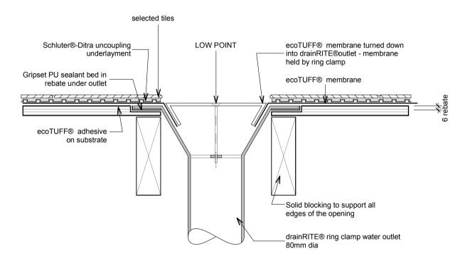
ecoT35 - drainRITE® Water Outlet 2 - ring clamped
