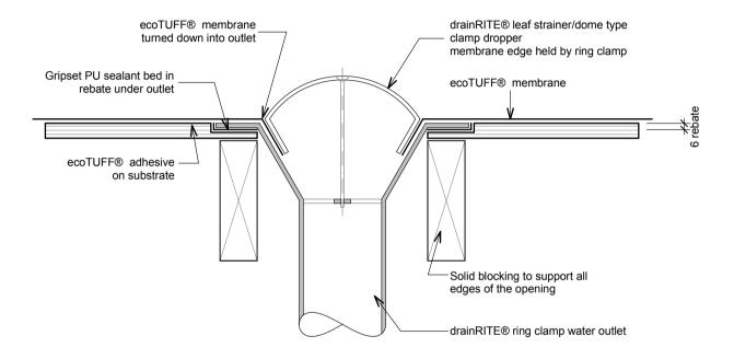
ecoT36 - drainRITE® Water Outlet 3 - ring clamped dome
