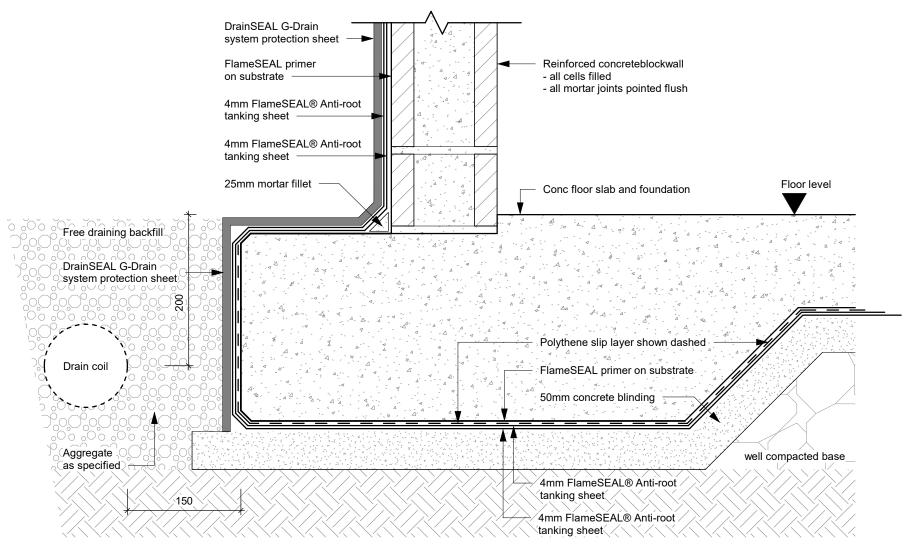
fS-T D12 - Blockwall/ Floor Joint 2-1 (Two Layer)
