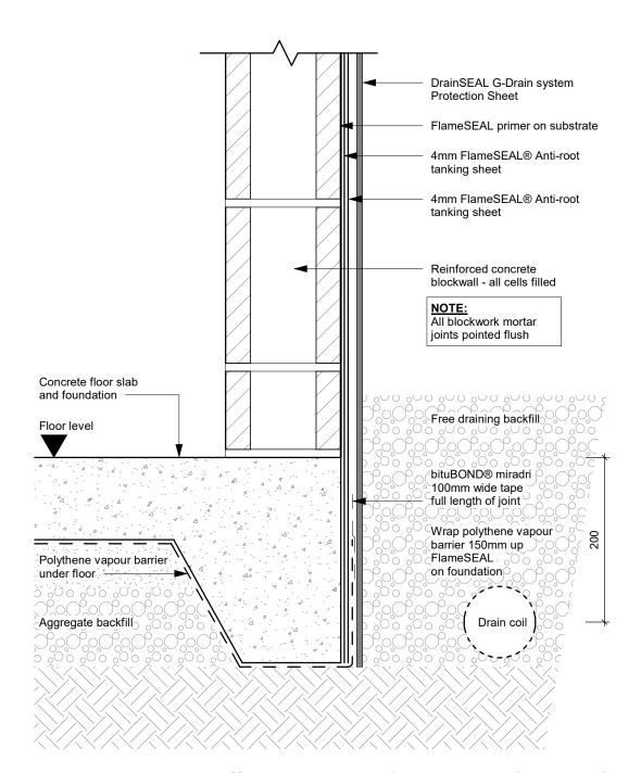
fS-T D14 - Blockwall/ Floor Joint 2-3 (Two Layer)
