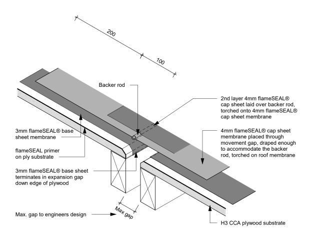
fS D02 - Ply Substrate Expansion Joint
