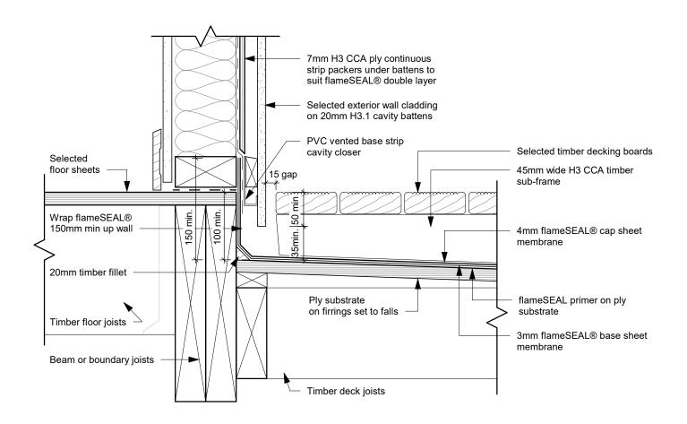
fS D35 - Timber Raft Floating Deck - Wall Detail - Type 1
