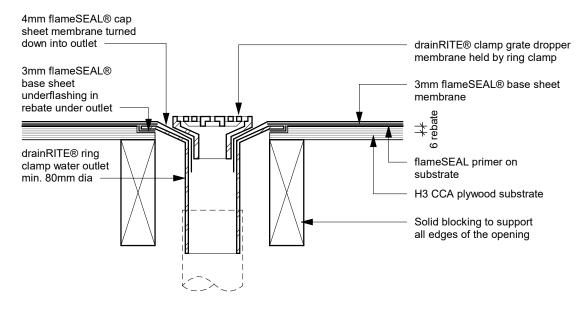
fS D26 - drainRITE® Water Outlet 1 - Ring Clamped Revision: 10 September 2019
