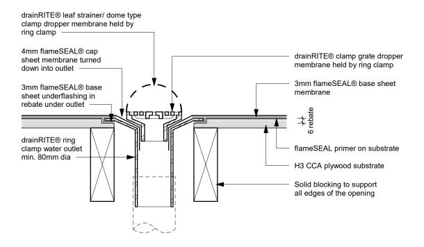
fS D27 - drainRITE® Water Outlet 2 - Ring Clamped Dome Revision: 10 September 2019
