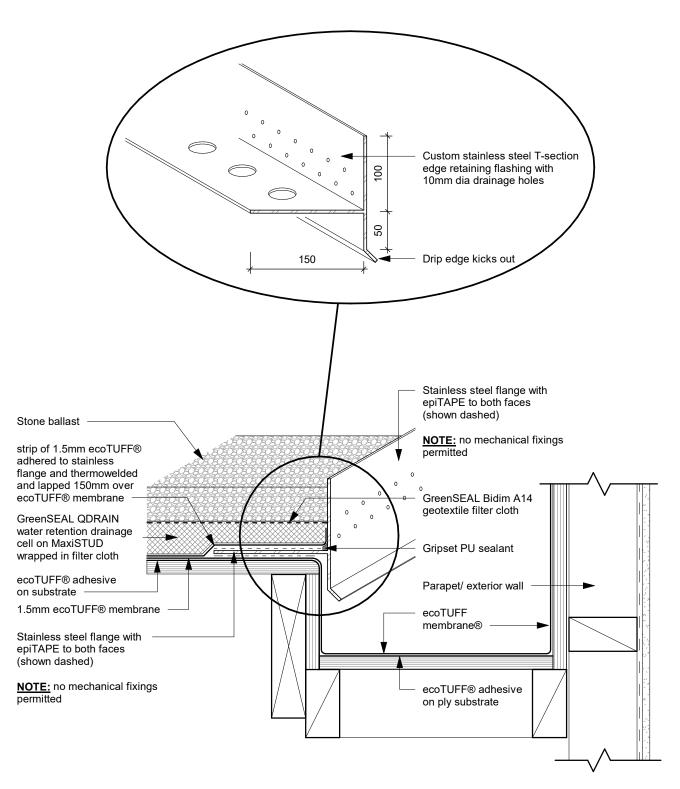
eT D04 (TPO) - Ballast Gutter
