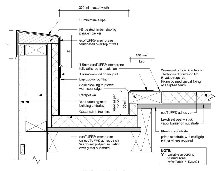
WS ET027 - Gutter Parapet
