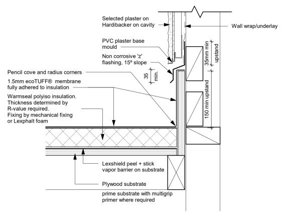
WS ET025 - Gutter Wall 1 - Cladding over Cavity
