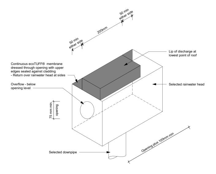
WS ET011 - Rainwater Head Scupper Outlet Revision: 28 June 2019
