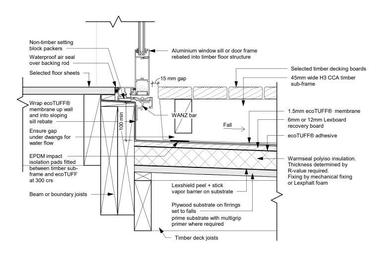
WS ET035 - Timber Raft Floating Deck - Threshold Detail - Type 1
