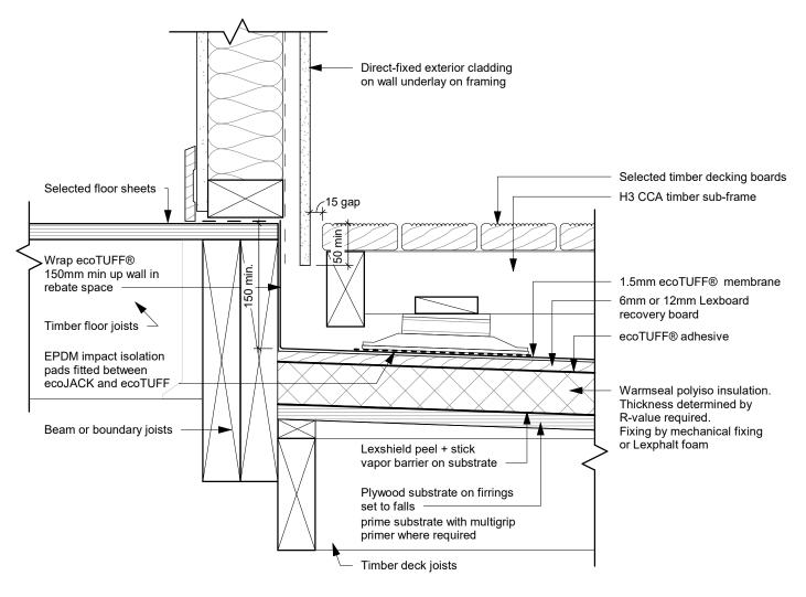
WS ET033 - Timber Raft Floating Deck - Wall Detail - Type 2
