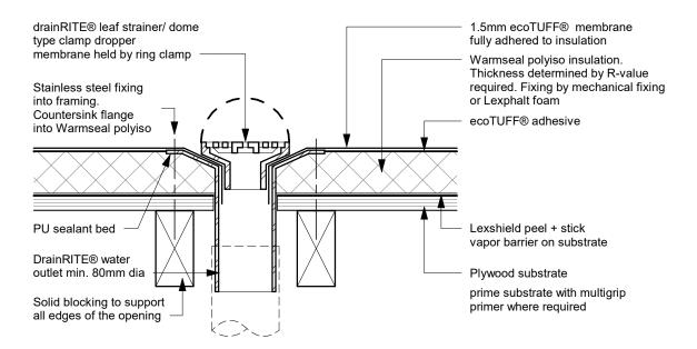
WS ET019 - drainRITE® Water Outlet 2 - Ring Clamped Domed
