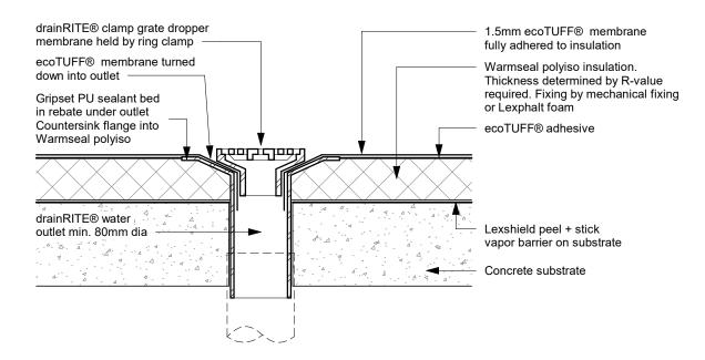
WS ET020 - drainRITE® Water Outlet 3 - Ring Clamped Domed
