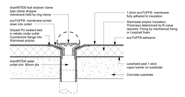
WS ET021 - drainRITE® Water Outlet 4 - Ring Clamped Domed
