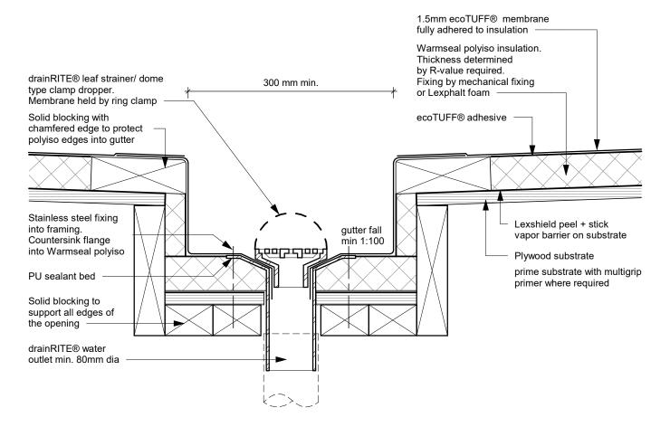
WS ET021 - drainRITE® Water Outlet 5 (Dropper) - Ring Clamped Dome Revision: 28 June 2019
