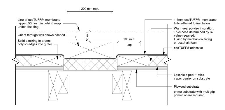
WS ET010 - Overflow Scupper Section 2
