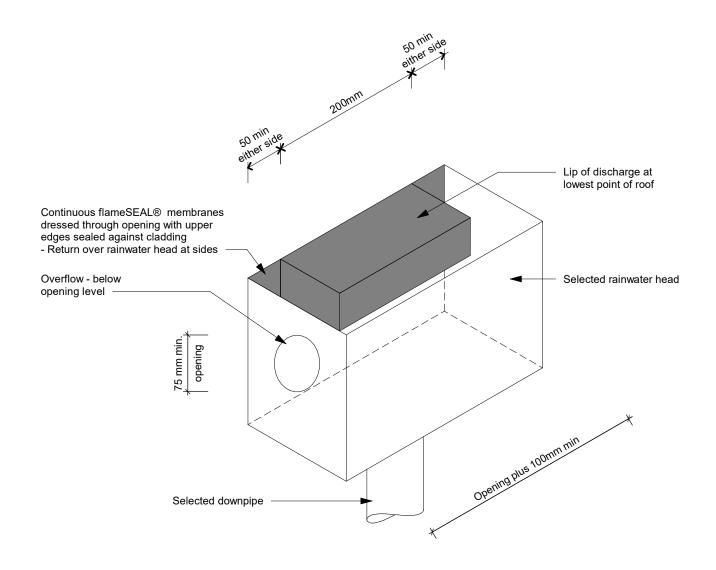
WR fS D11 - Rainwater Head Scupper Outlet
