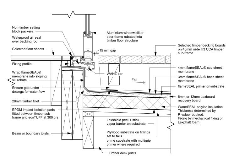
WR fS D35 - Timber Raft Floating Deck - Threshold Detail - Type 1
