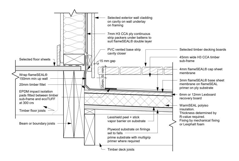
WR fS D33 - Timber Raft Floating Deck - Wall Detail - Type 1
