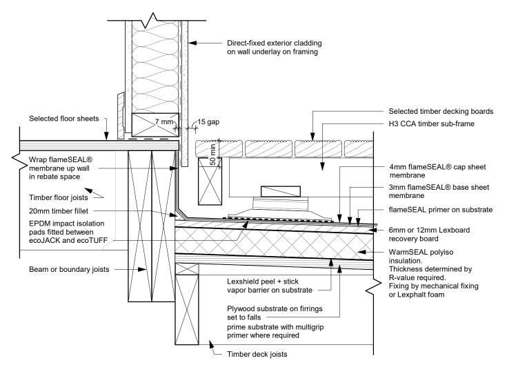
WR fS D34 - Timber Raft Floating Deck - Wall Detail - Type 2
