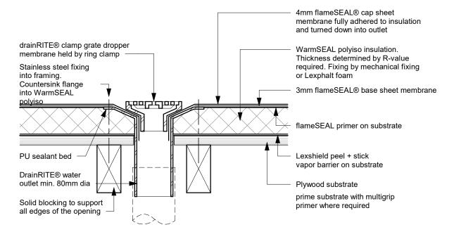
WR fS D18 - drainRITE® Water Outlet 1 - Ring Clamped Revision: 10 September 2019
