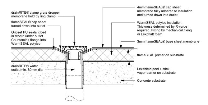
WR fS D20 - drainRITE® Water Outlet 3 - Ring Clamped Domed
