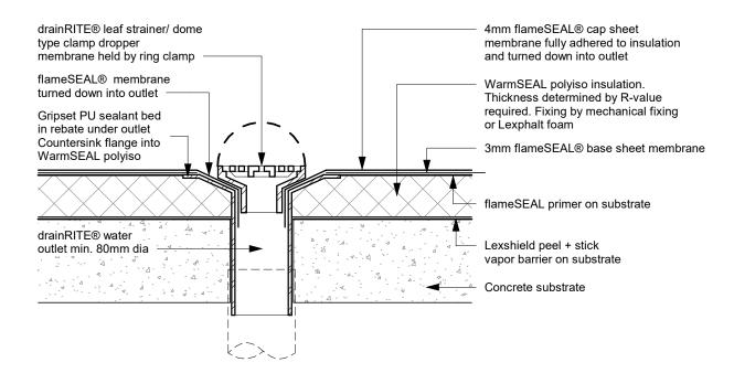
WR fS D21 - drainRITE® Water Outlet 4 - Ring Clamped Domed
