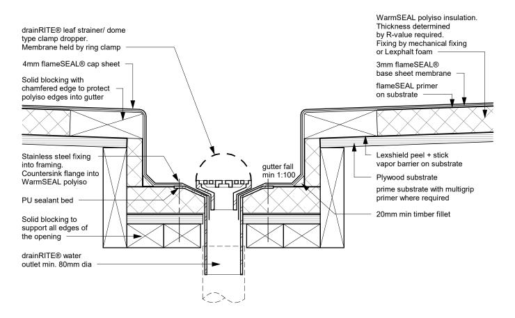
WR fS D22 - drainRITE® Water Outlet 5 (Dropper) - Ring Clamped Dome Revision: 10 September 2019
