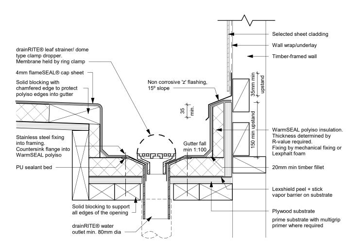
WR fS D23 - drainRITE® Water Outlet 6 (Dropper) - Ring Clamped Dome
