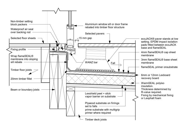
WR fS D32 - ecoJACK® Paver - Threshold Detail - Type 1
