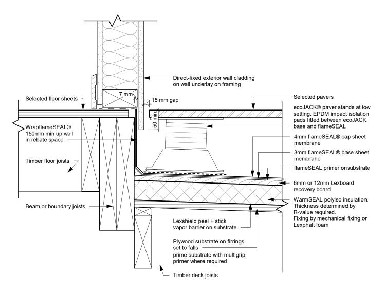
WS ET031 - ecoJACK® Paver - Wall Detail - Type 2
