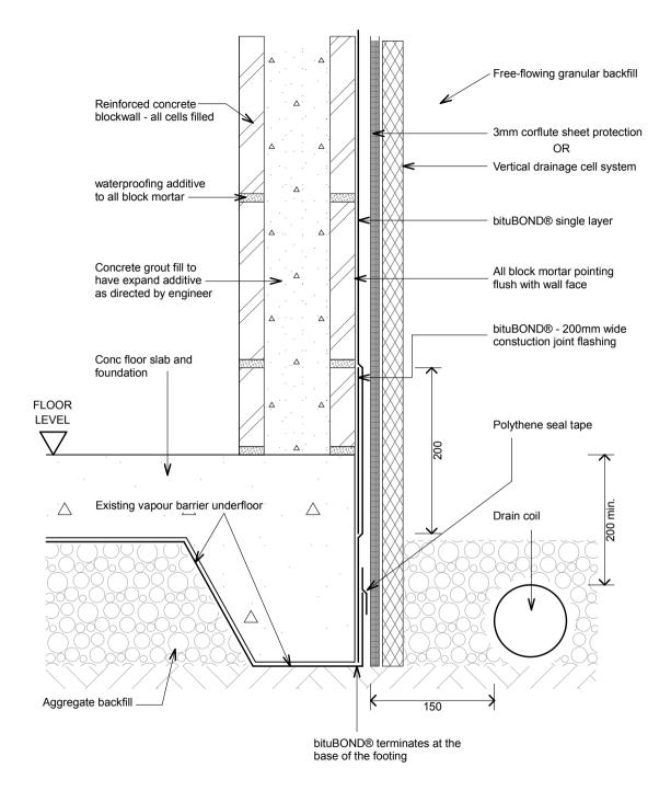
bitu-B13 - Blockwall Foundation type 1
