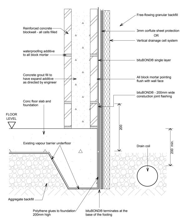
bitu-B23 - Blockwall Foundation type 2
