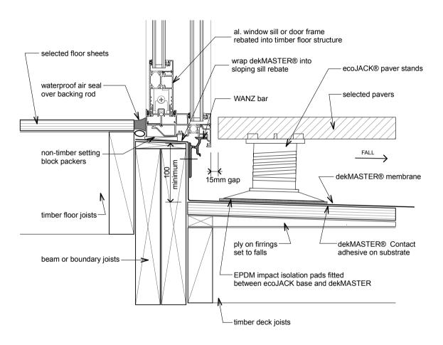
dek-M34 - ecoJACK® paver-threshold detail - type 1
