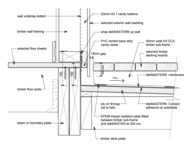
dek-M36 - timber raft floating deck-wall detail - type 1
