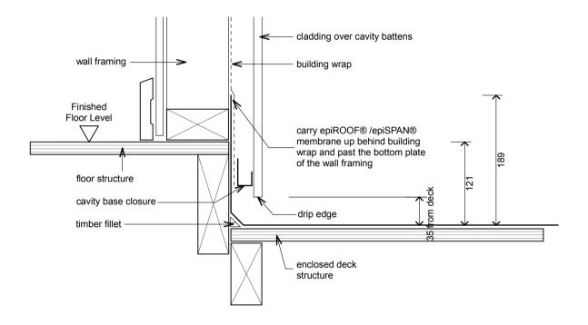
epiD03 - Deck Detail 3 - Cavity Wall Base
