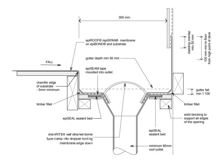
epiD06 - drainRITE® Deck Drain Type 2
