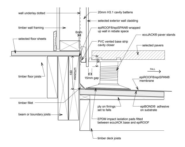
epiD09 - ecoJACK® paver-wall detail - type 2
