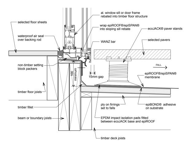
epiD10 - ecoJACK® paver-threshold detail - type 1
