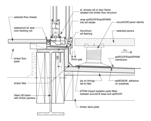
epiD11 - ecoJACK® paver-threshold detail - type 2
