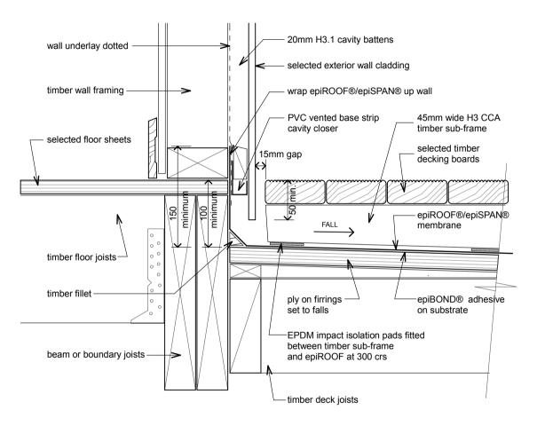
epiD12 - timber raft floating deck-wall detail - type 1
