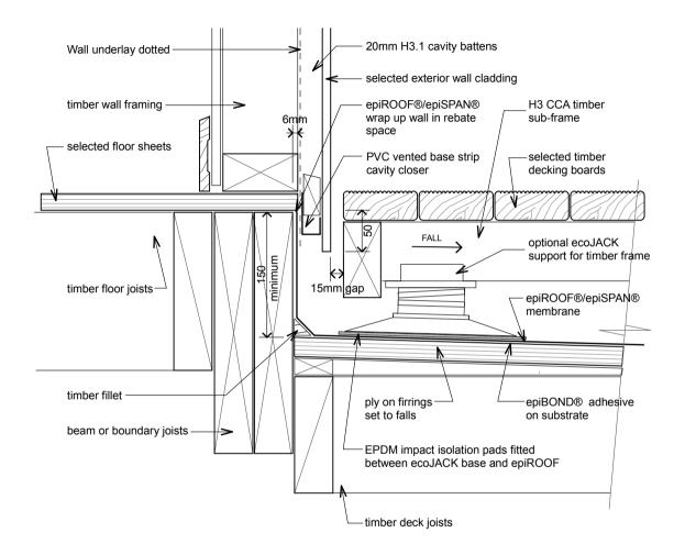
epiD13 - timber raft floating deck-wall detail - type 2
