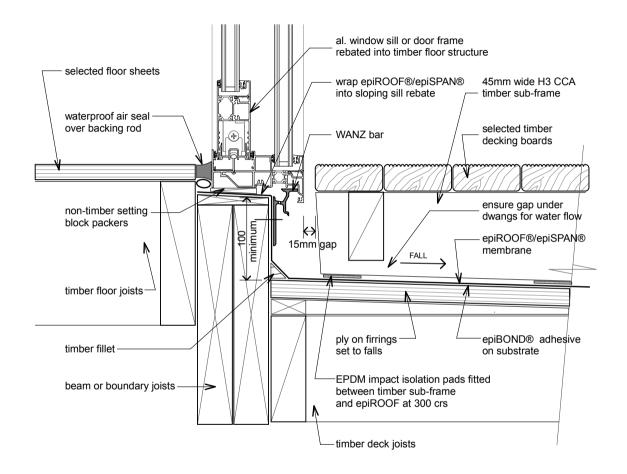
epiD14 - timber raft floating deck-threshold detail - type 1
