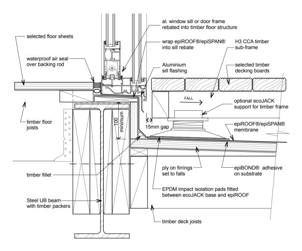
epiD15 - timber raft floating deck-threshold detail - type 2
