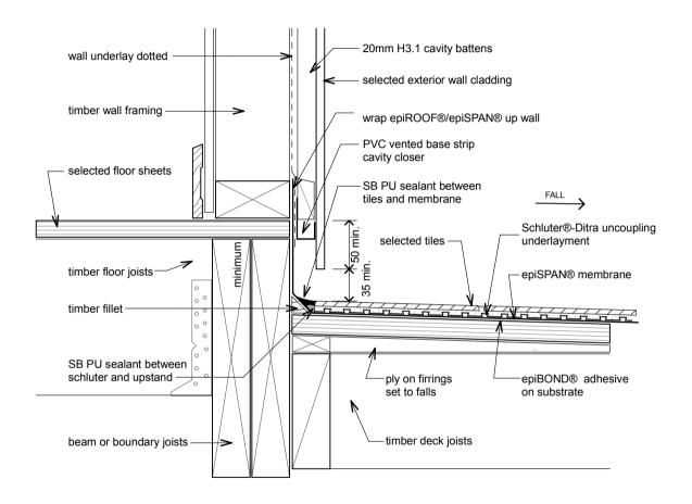
epiD16 - Tiles (on Uncoupling underlay)-wall junction
